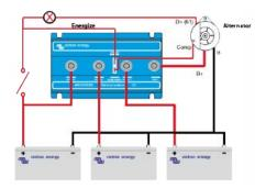
Features: • Low voltage drop due to the use of high efficiency Schottky diodes • Various models available with 2 or 3 outputs and alternator energise connection
