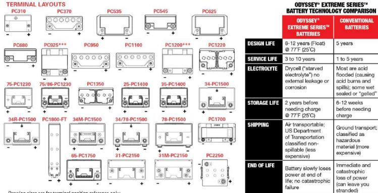
Drawing sizes are for terminal position reference only; diagrams are not proportionate to each other. \*\*\*Optional Reversed Polarity (L)
