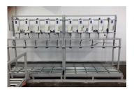
Combined charger stands and roller beds are easily the best solution for lateral changing of batteries. The design combines the best features of standard charger frames and roller beds into one compact unit.
