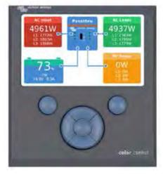
Color Control Panel, showing a PV application
