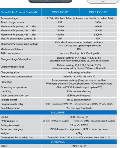
1a) If more PV power is connected, the controller will limit input power to the stated maximum.
