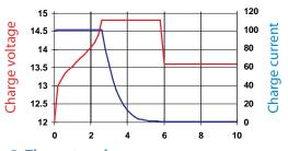
Fig. 3: Three step charge curve
