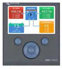
Color Control panel, showing a PV application
