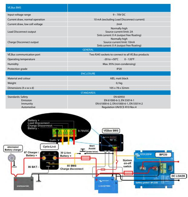
Figure 2: Application example for a vehicle or boat, without inverter/charger.
