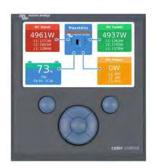
Color Control panel, showing a PV application
