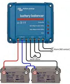
Battery Balancer connected to two series connected 12V batteries (24V system)
